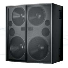
The PSW-6 high-power cardioid subwoofer is the first low-frequency system to exhibit a true cardioid directional pattern throughout its operating range. The PSW-6's unprecedented directional control spans more than two full octaves, with a front-to-back SPL ratio of more than 15 dB (typically 20 dB) from 30 Hz to 125 Hz. Horizontal and vertical coverage patterns are symmetrical, ensuring consistent SPL and frequency response throughout the coverage area.
