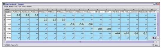
Each Galileo output can receive a separate mix of the six inputs.
