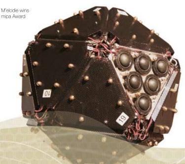
Meyer Sound's collaboration with the University of California, Berkeley includes CNMAT's spherical loudspeaker array.
