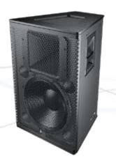
The UPQ-2P is a self-powered two-way loudspeaker designed for applications requiring high acoustic power output, extremely low distortion, and a narrow symmetrical coverage pattern with predictable characteristics. The UPQ-2P's compact, vented enclosure houses a 15-inch neodymium magnet low/mid driver, a 4-inch diaphragm compression driver coupled to a conical high frequency horn, and a two-channel amplifier with a total peak output power of 1275 watts. Maximum peak SPL measures 136 dB at 1 m.
